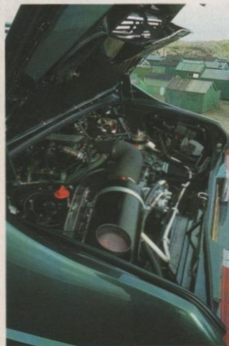
Rear-mounted 3.5-litre V8 engine (left) pumps out 220bhp at 5750rpm and 224lb ft at 3500rpm. Tatra claims a top speed of 138mph and 0-60mph in a sprightly 7.7sec. Large, deep side windows provide good visibility, but look a little ungainly (below)
